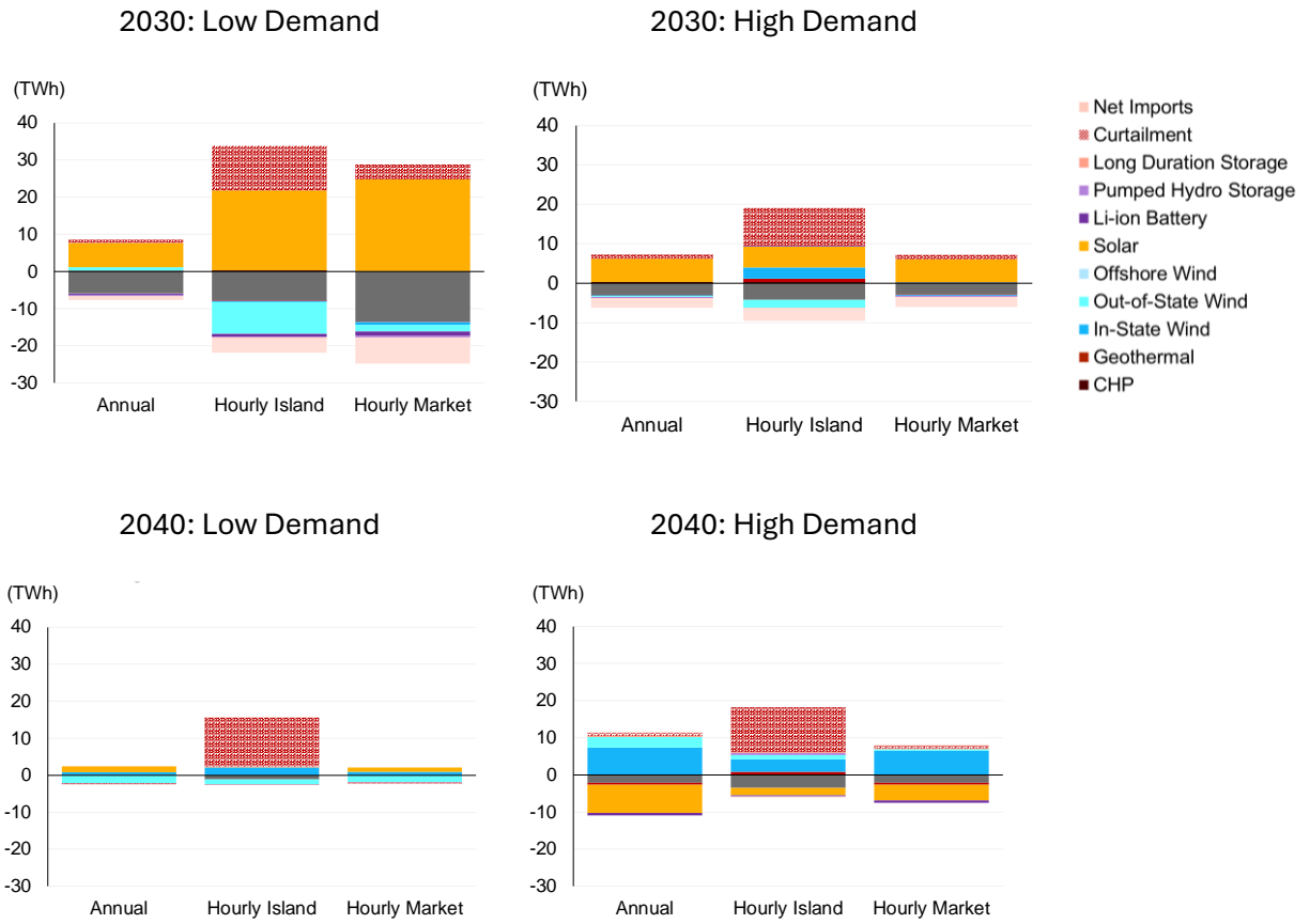
Figure A-5. CAISO-wide Generation Changes in Annual and Hourly Matching in 2030 and 2040 for 25% C&I Matching under Low Demand and High Demand Scenarios
